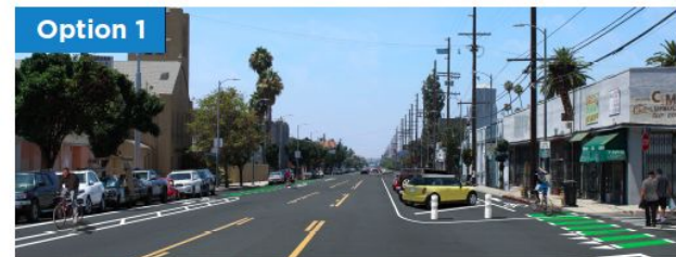
Angled parking on north side of street with protected bike lane (westbound) and standard bike lane with safety buffer (eastbound).
